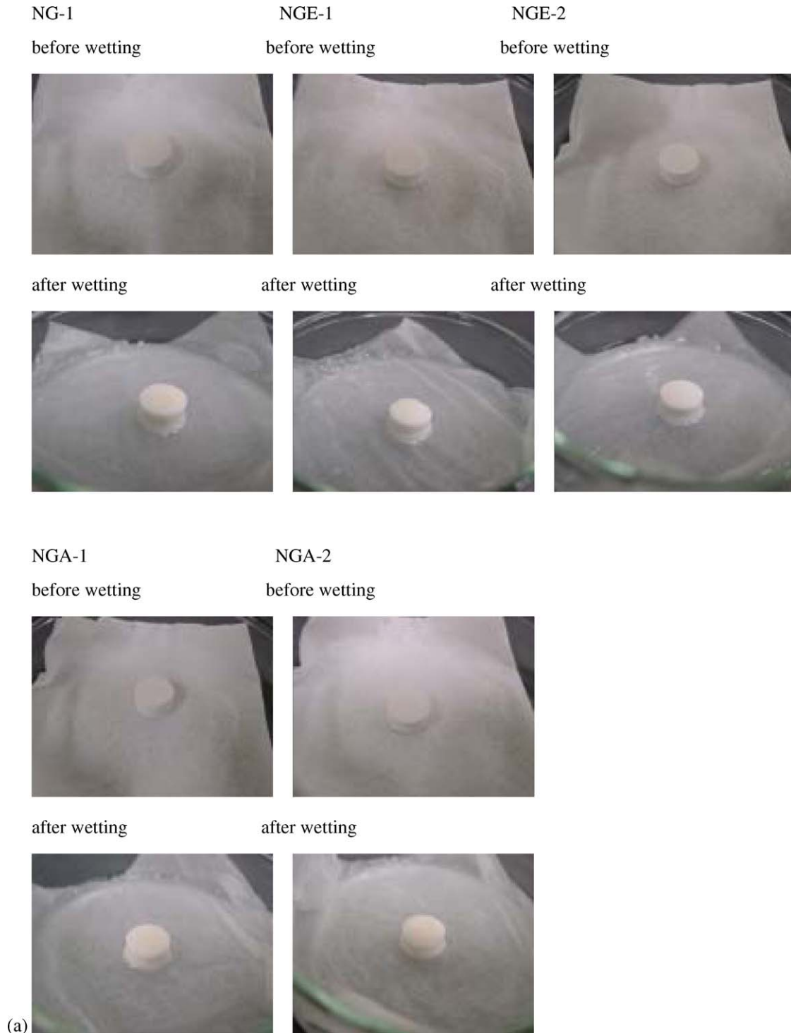
Fig. 8. (a) Change in the appearance of the tablets as formulated in Table 2 by wetting. (b) Effect of ethenzamide on the disintegrating property: (●) NS-300 and glycine, (□) 20% and (◇) 10%. Data are expressed as means ( n=5 ). (c) Effect of ascorbic acid on the disintegrating property: (●) NS-300 and glycine, (□) 20% and (◇) 10%. Data are expressed as means ( n=5 ).
